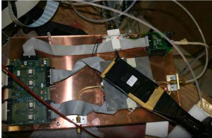
**Figure 3.68:** Experimental setup for the small high-resistivity bakelite RPC.
