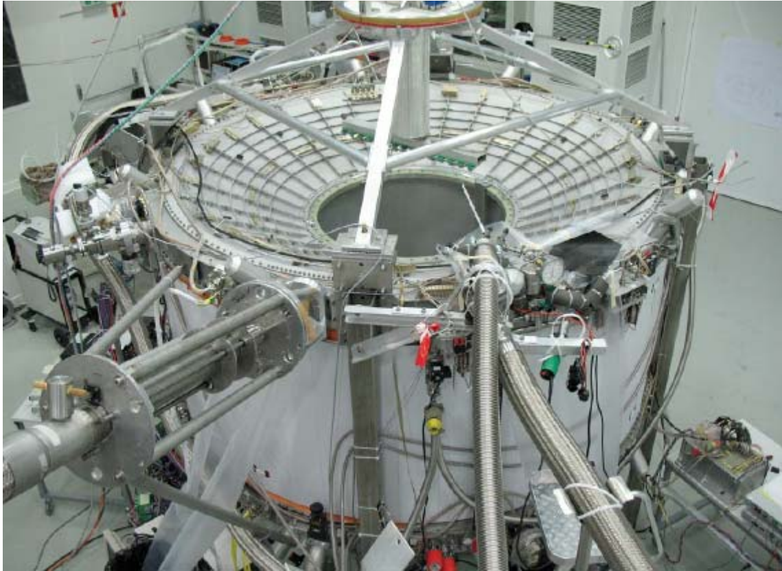
Fig. 2.12 The AMS-02 superconducting magnet during the tests at CERN
