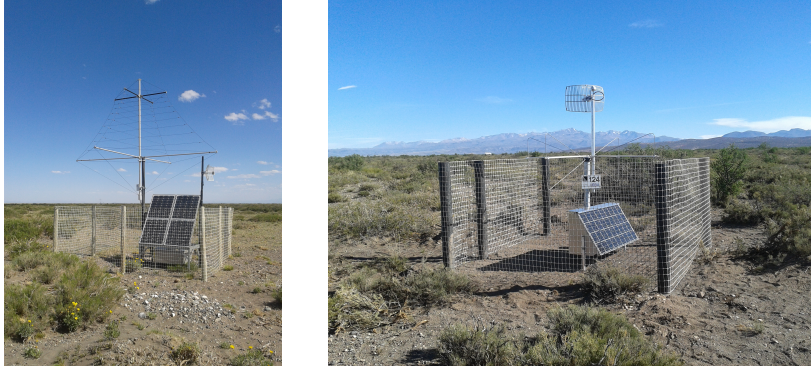
Figure 2: Photos of the AERA radio stations a) logarithmic periodic dipole radio station b) butterfly radio station. The butterfly antenna is located underneath the parabolic wifi antenna.
