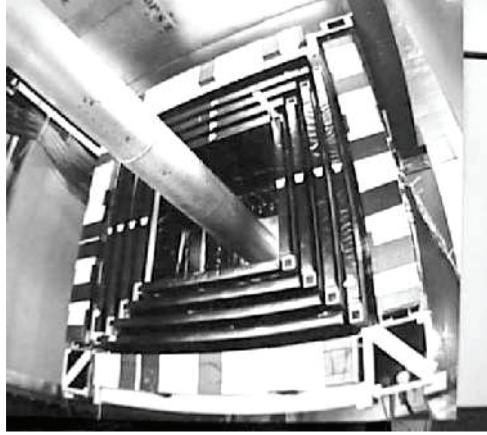
Figure 1: Photo of the early CUSB detector with the CESR beam pipe and the four square layers of NaI crystals.
