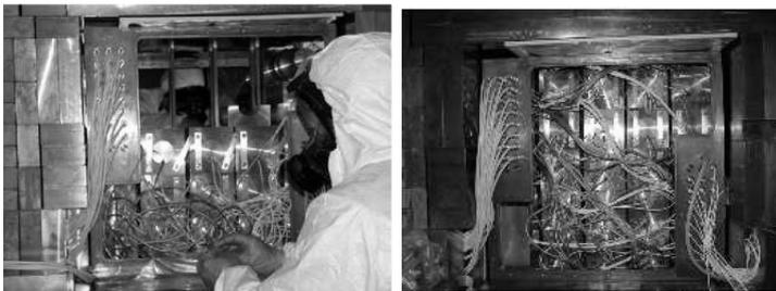
Figure 8: Left: *the installation of the 25 NaI(Tl) crystals (9.70 kg each one) of DAMA/LIBRA in HP Nitrogen atmosphere. Right: One of the final stages of the detectors' installation. All the procedures as well as these photos have been carried out in HP Nitrogen atmosphere.*
