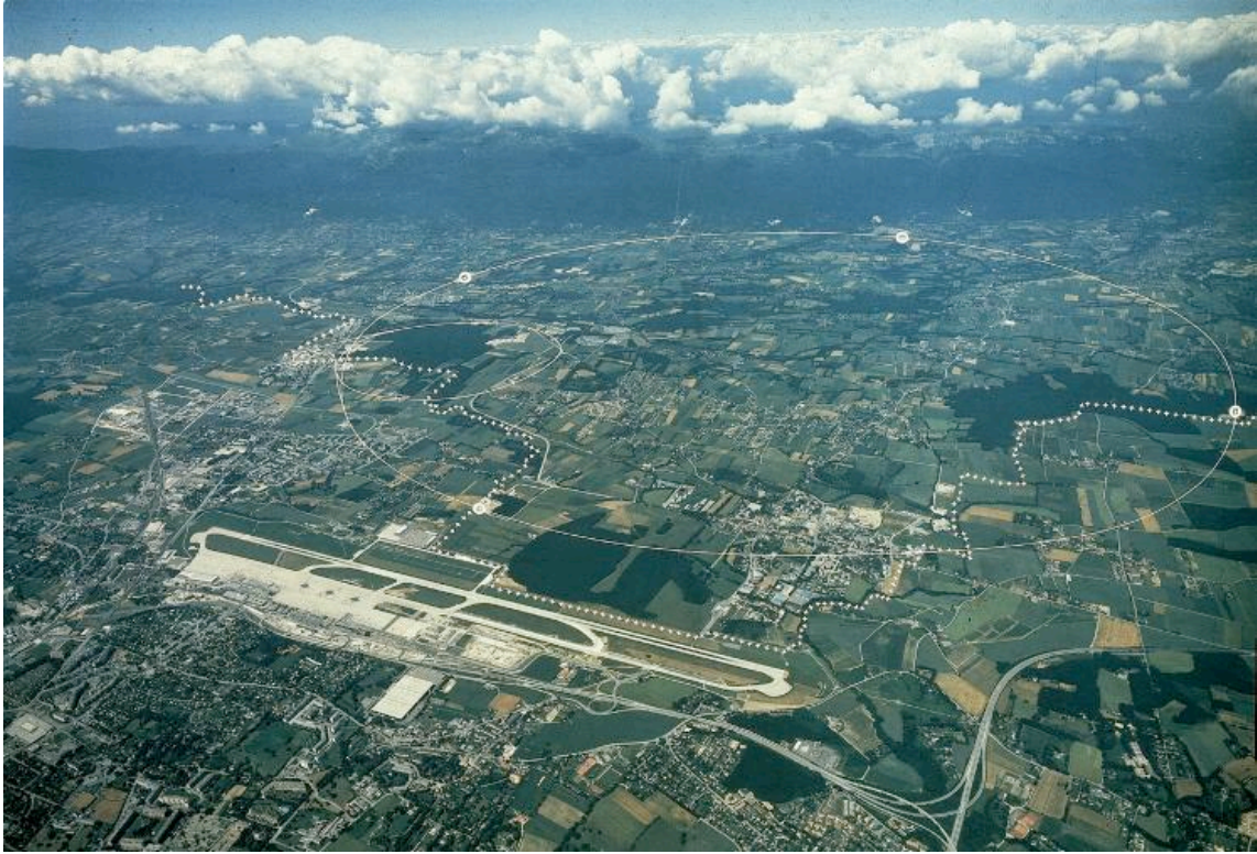
Aerial view of the CERN site just outside Geneva, Jura mountains in the background. The large circle shows the line of the LEP tunnel, 27 km in circumference. The small circle shows the SPS tunnel, 7 km in circumference. The border line indicates the Franco-Swiss border (1987).
