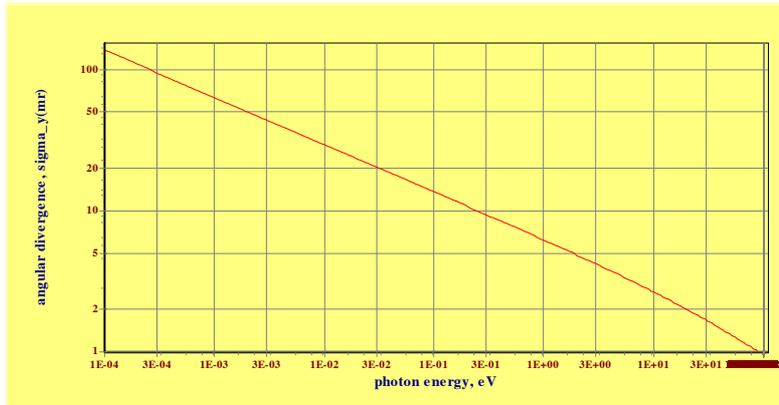
Figure 6: *Photon beam divergence from a DAΦNE dipole magnet.*
