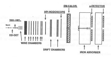
Figure 1: Schematic view of the WA92 setup.
