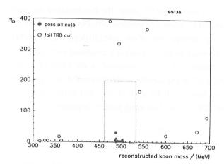
Fig. 6: Reconstructed invariant kaon mass of  $K_L \rightarrow e^+e^-e^+e^-$  candidates vs. the quantity  $d^2$  from the vertex fit. Solid (open) circles are events which pass (fail) the TRD electron identification cut.
