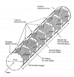
Figure 8: Liquid krypton calorimeter prototype.
