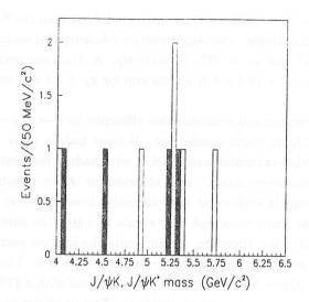
Figure 5: Combined  $J/\psi + K^{\pm}$  and  $J/\psi + K^{0*}$  invariant mass; the shaded entries are  $J/\psi K^{\pm}$  combinations.
