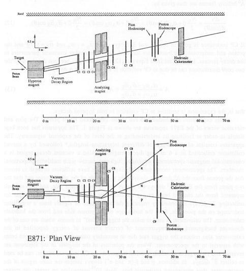
Figure 1. Plan and elevation views of E871 spectrometer
