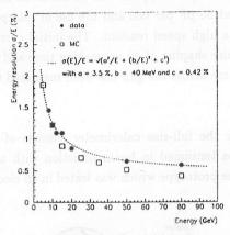
Figure 9: Energy resolution of the liquid krypton calorimeter prototype.
