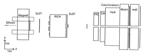
Figure 1: Layout of "existence-proof" spectrometer (bend view).
