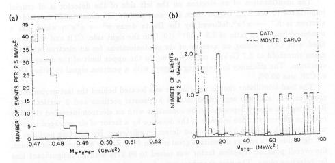
Figure 3. (a) Invariant mass distribution of  $M_{\pi ee}$  for  $M_{ee} \leq 15 \text{MeV/c}^2$ . (b)  $M_{\pi ee}$  distribution for 492.5 MeV/c<sup>2</sup>  $\leq M_{\pi ee} \leq 520$  MeV/c<sup>2</sup>. The dashed line indicates the signal expected from the decay of a 1.8 MeV/c<sup>2</sup>  $A^0$  with a branching ratio  $BR(A^0 \to e^+e^-) = 10^{-6}$ . The high mass tail on this distribution results from electron bremsstrahlung and multiple Coulomb scattering.
