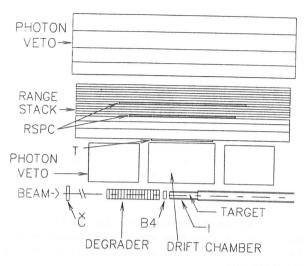
Figure 3: Side view of the E787 detector. Only the top half of the detector is shown. The detector has cylindrical symmetry.
