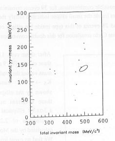
Fig. 9: Invariant  $(\gamma \gamma e^+ e^-)$ -mass vs. invariant  $\gamma \gamma$  mass for  $K_S \to \pi^0 e^+ e^-$  candidates. The ellipse indicates a  $3\sigma \times 3\sigma$  signal region.
