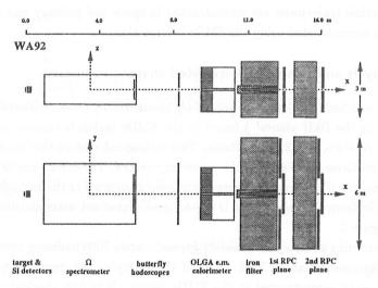
Figure 1: Schematic view of the WA92 setup.
