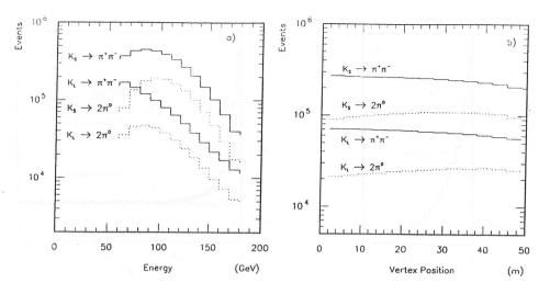
Figure 3: Measured energy spectra (a) and vertex distributions (b).
