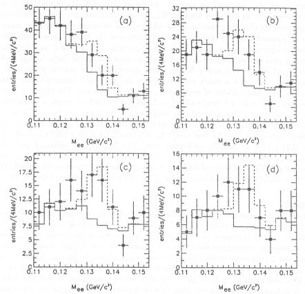
Figure 9.  $M_{ee}$  distributions in the vicinity of the  $\pi^0$  for  $M_{\pi ee} < 0.504~GeV/c^2$  and (a)  $M_{\pi ee} > 0.483~GeV/c^2$ , (b)  $M_{\pi ee} > 0.487~GeV/c^2$ , (c)  $M_{\pi ee} > 0.490~GeV/c^2$  and (d)  $M_{\pi ee} > 0.492~GeV/c^2$ . The solid histogram is the Monte Carlo simulation with no  $\pi \to e^+e^-$ . The dashed histogram indicates the fit of the peak finding program.
