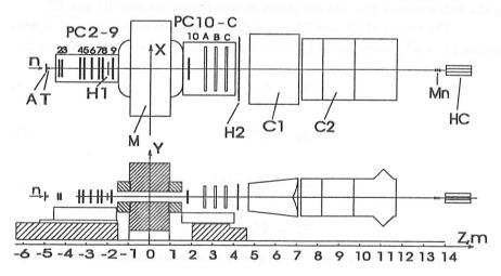
Figure 2: Arrangement of the EXCHARM spectrometer elements at the 5N channel of the Serpukhov accelerator: n - neutron beam; A - anticoincidence counter; T - target; M - magnet; PC - multiwire proportional chambers; H1,H2 - scintillation hodoscopes; C1,C2 - Cherenkov threshold counters; Mn - neutron monitor; HC - hadron calorimeter
