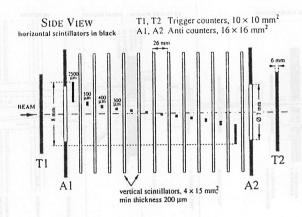
Figure 7: The proton tagging counter.
