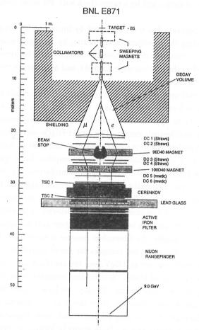
Figure 8: The E871 apparatus.
