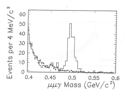
Figure 1:  $\mu^+\mu^-\gamma$  mass distribution after cuts. Histogram is data for events with  $P_t^2$  less than 200  $MeV^2/c^2$  and points are for events with  $P_t^2$  greater than 200  $MeV^2/c^2$  and less than 1000  $MeV^2/c^2$  normalized to the low  $P_t^2$  data.
