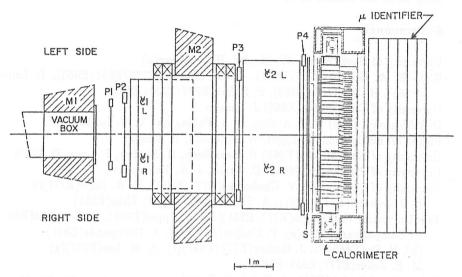
Figure 10. The E865 Apparatus.
