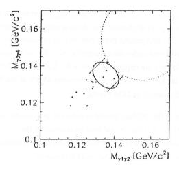
Fig. 11: Two-photon masses for the 16  $K_L \to \pi^0 \pi^0 \gamma$  candidate events that pass all cuts. The signal region for  $\pi^0 \pi^0 \gamma$  events is shown as solid ellipse. The curve from fig. 10 encircling the background events from  $3\pi^0$  is the light-dashed curve. Three events lie within the signal region.
