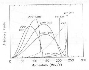
Figure 2: Momentum spectrum for charged particles from  $K^+$  decay. Branching ratios are given in parentheses.
