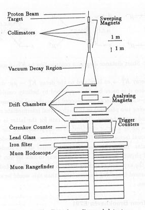
Figure 3: The E791 beamline and detector.
