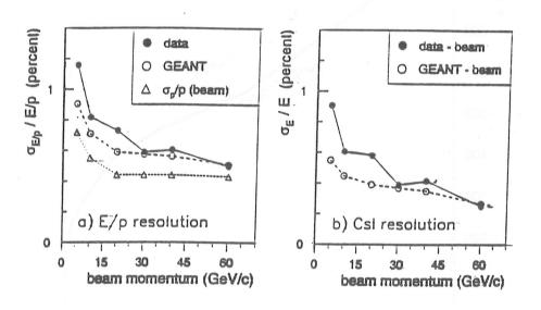
Figure 3: a) \*PRELIMINARY\* E/p resoultion .vs. beam momentum, and b) the intrinsic CsI resolution with the beam contribution subtracted.
