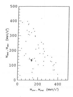
Fig. 8: Scatter plot of the two possible combinations of invariant photon-electron masses for  $KS \to \pi^0 e^+ e^-$  candidate events (two entries/event). Entries inside the ellipse are due to  $\pi^0 \pi^0$  events with double conversion.
