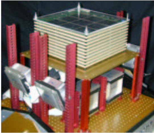
Figure 3: *The MEGA prototype detector during a preliminary stage of completion. The tracker consists of 10 layers and 4 calorimeter blocks are visible.*
