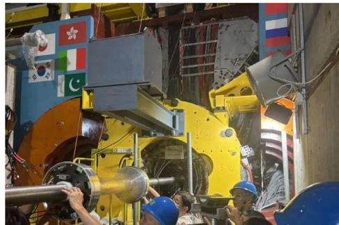
Figure 2: Left picture: the mechanical team with a CGEM mockup after a successful insertion test. Right picture: the inner drift chamber extracted from BESIII, to leave space for the CGEM-IT.
