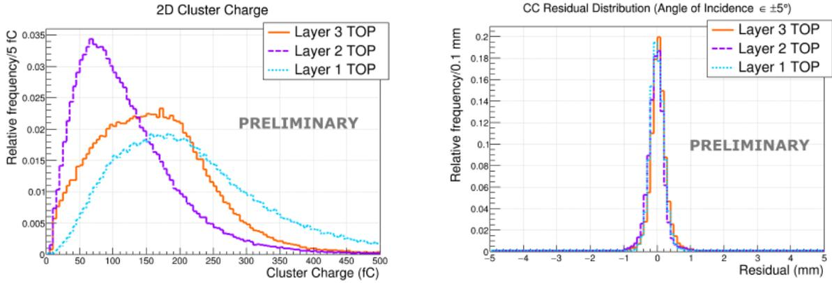
Figure 1: Preliminary results on cosmic ray data: on the left the charge of 2D clusters obtained combining neighboring hits in both views, on the right the exclusive residuals distribution for almost perpendicular tracks.
