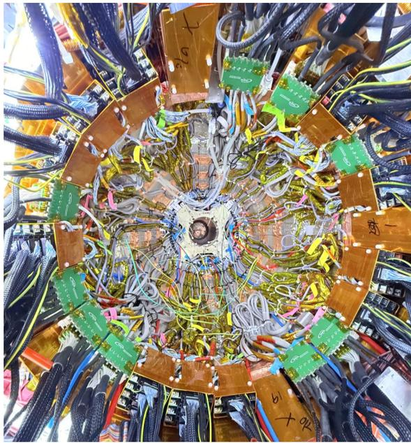
Figure 3: Some pictures of the CGEM installation inside BESIII: positioning in front of the insertion hole (top left), slowly going inside (top middle), reaching the final position, front view with electronics and cabling (bottom).
