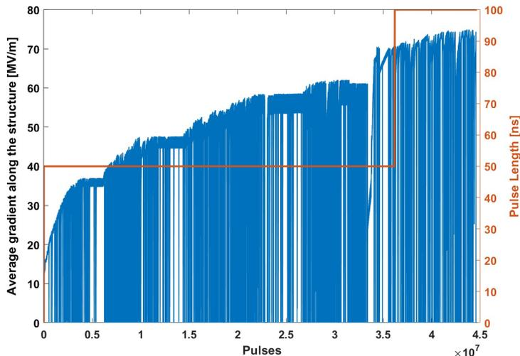
Figure 3: *Conditioning history of the EuPRAXIA@SPARC\_LAB 20 cells RF prototype*
