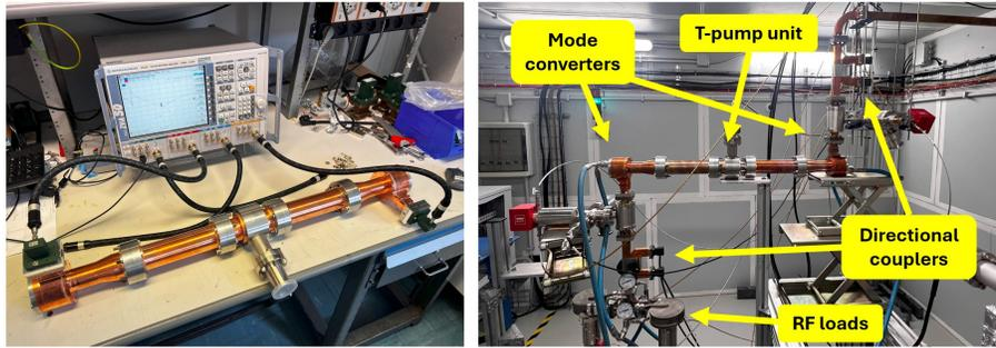
Figure 1: *Mode converter and circular waveguide setup during low-power testing after manufacturing (left), and layout of the circular waveguide setup during high-power testing inside the TEX bunker (right).*
