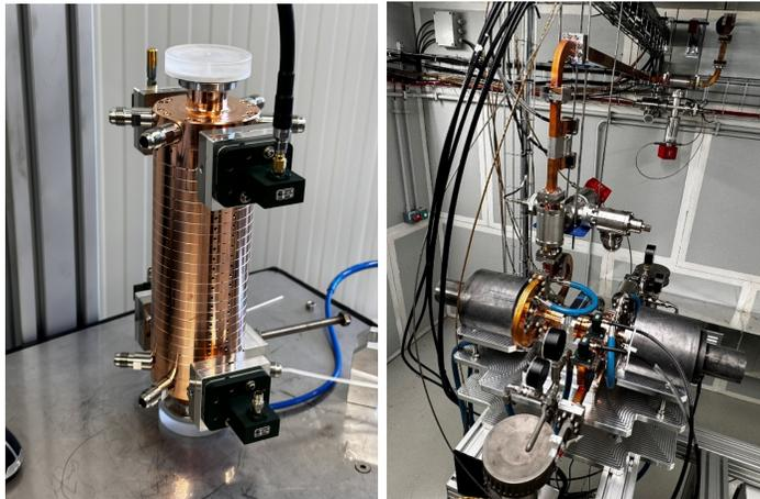
Figure 2: *X-band 20 cells RF prototype of the EuPRAXIA@SPARC-LAB structure (left) and high power test layout of the structure inside the TEX bunker (right).*
