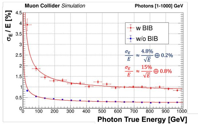
Figure 1: Simulated energy resolution in the Muon Collider framework with and without BIB contributions.
