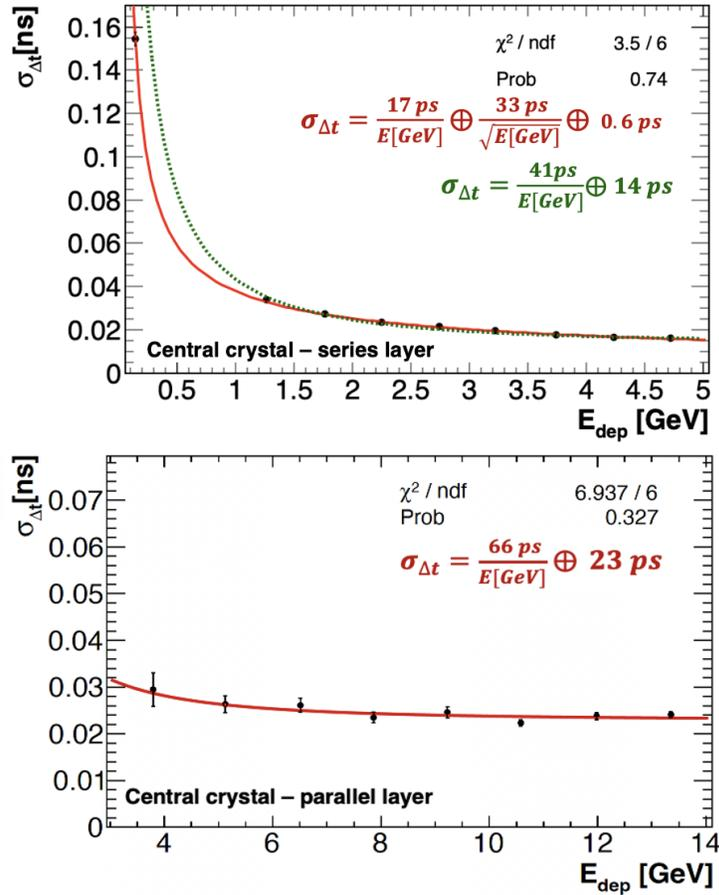
Figure 2: Time resolution as a function of the energy deposited in the crystal with the highest energy deposit. A time resolution measurement with a 450 MeV electron beam was added for the series layer (solid red line fit).
