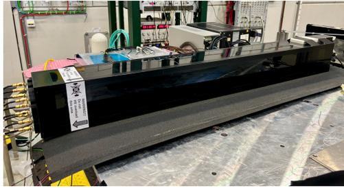
Figure 8: Prototype shashlyk module for the HIKE Main Electromagnetic Calorimeter during beam tests at the CERN PS in September 2024.
