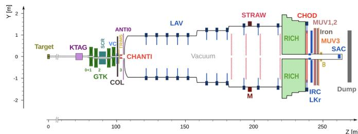
Figure 1: Schematic view of the NA62 experiment, showing the kaon production target, KTAG Cherenkov  $K^+$  beam tagger, GTK beam tracker, CHANTI collar veto, LAV large-angle photon vetoes, STRAW straw-tube trackers, RICH ring-imaging Cherenkov detector, CHOD hodoscope, MUV1-3 hadron calorimeters and muon vetoes, LKr calorimeter, and IRC and SAC small-angle photon vetoes.
