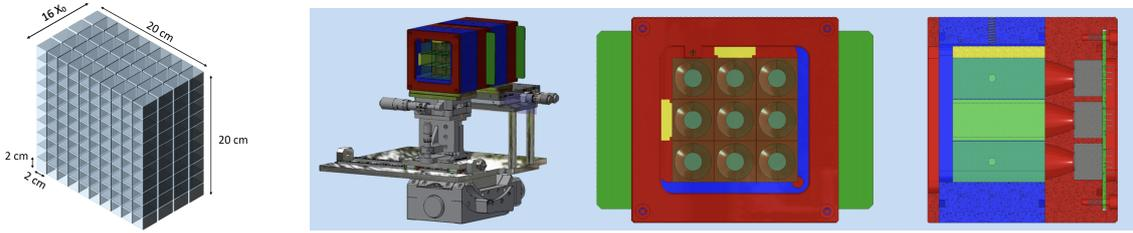
Figure 7: Left: Dimensional sketch of a SAC based on dense, high- $Z$  crystals with both transverse and longitudinal segmentation. Right: Mechanical designs for HIKE SAC prototype. From left to right: complete assembly, including mechanics for relative positioning and angular rotation between layers; front view, sectional side view showing Winston cones and PMTs.
