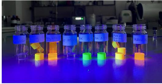
Figure 9: Conventional scintillator, nanocomposite scintillator, and control samples for light yield measurements at the Frascati BTF and CERN PS, seen under ultraviolet light.
