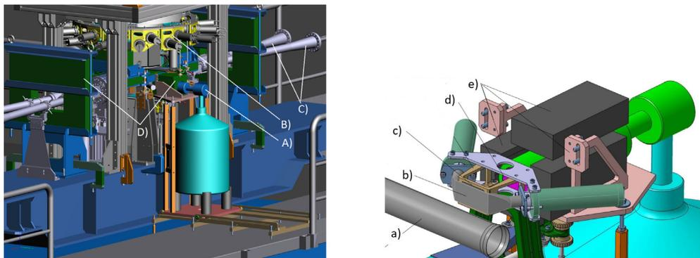
Figure 7: The location of the HPGe detector in the SIDDHARTA-2 setup, left: A) the HPGe detector, B) the SIDDHARTA-2 setup, C) beam pipes, D) shielding. Details of the HPGe setup, right: a) beam pipe, b) scintillation detector SC1, c) lead target, d) active part of the HPGe detector, e) lead shielding with holder (reported from <sup>16</sup>).
