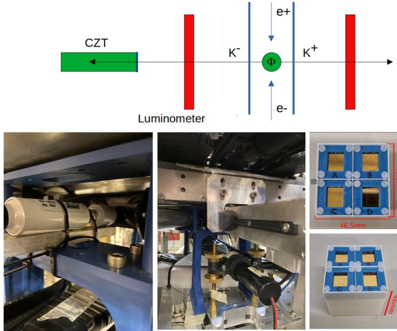
Figure 9: Top: Schematic of the main components for the two CZTe tests (not in scale) Bottom: picture of the installed RITEC CZT/500 detector (left), of the custom one (center) and of the unit cell installed in its aluminum box (right) (reported from <sup>17</sup>).
