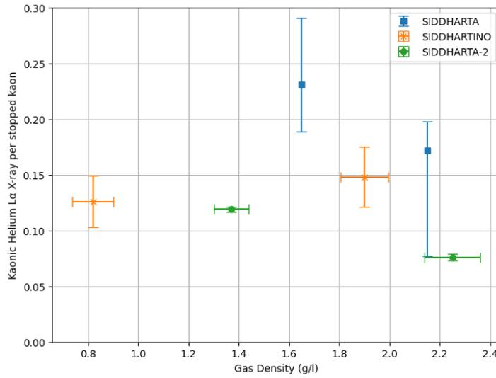
Figure 6: KHe-4  $L_\alpha$  yields as a function of the gas density. The increasing precision of the measurements is visible as the experiments were upgraded from SIDDHARTA <sup>7)</sup> (blue markers) to SIDDHARTINO <sup>11)</sup> (orange) and SIDDHARTA-2 <sup>13)</sup> (green) (reported from <sup>14)</sup>).
