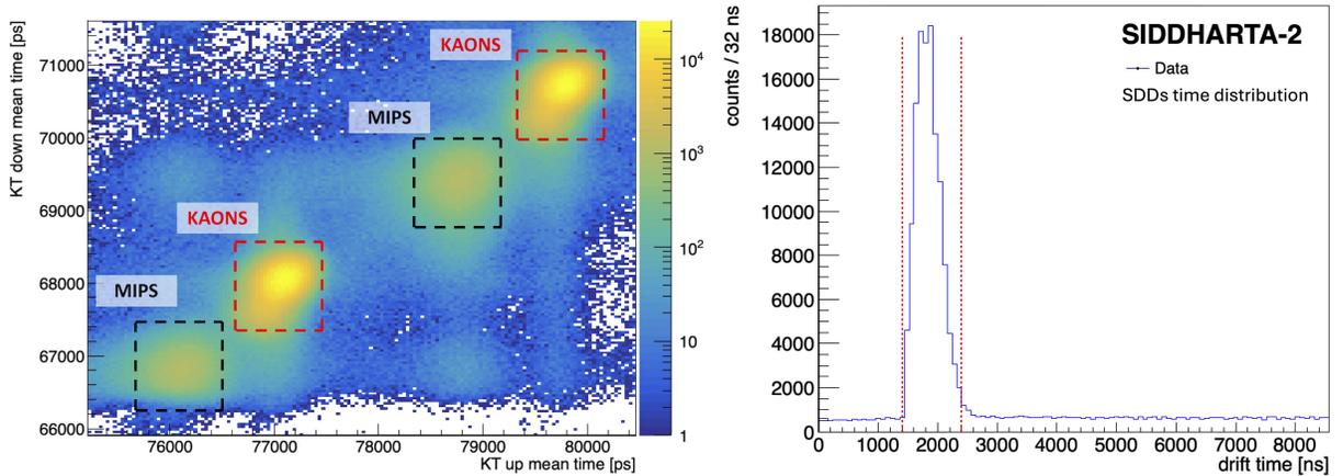
Figure 3: Left: Plot of the time difference between the kaon trigger top (KT up) and bottom (KT down) scintillators and the DAΦNE radio-frequency. The coincidence events related to kaons (high intensity) are clearly distinguishable from MIPS (low intensity). Right: Distribution of the time difference between the kaon trigger signals and X-ray hits on the SDDs. The dashed lines represent the  $1.0 \mu\text{s}$  acceptance window.
