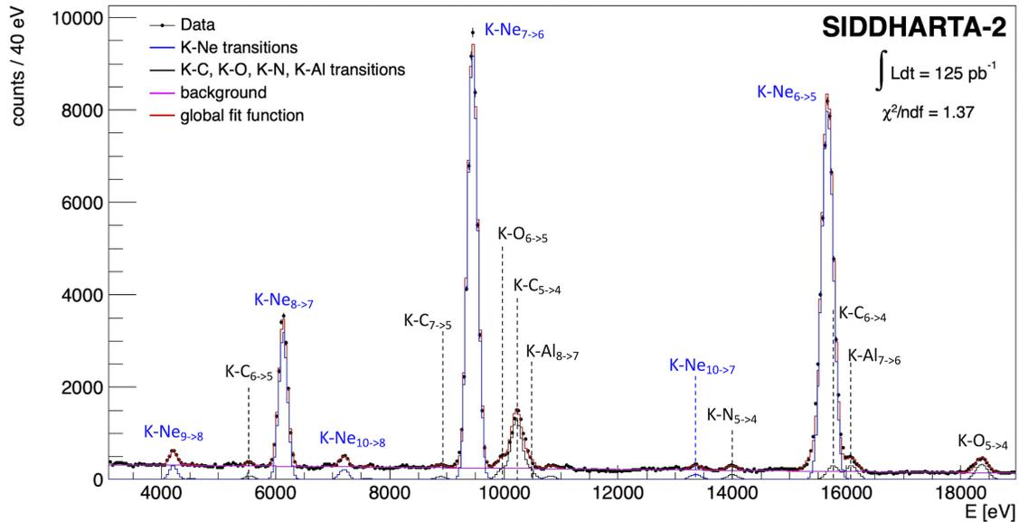
Figure 4: Kaonic Neon energy spectrum and relative fit after the events selection. The energy transitions are identified by the initial ( $n_i$ ) and final ( $n_f$ ) principal quantum numbers of the atomic levels. The several contributions of the fit function (red line) are highlighted: the kaonic neon (K-Ne) transitions in blue, the kaonic carbon (K-C), nitrogen (K-N), oxygen (K-O) and aluminium (K-Al) in black and the background in pink (reported from [15]).
