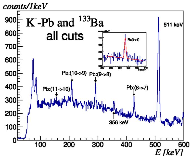
Figure 8: The spectrum seen by the HPGe detector after applying all cuts. The inset shows the peak at  $292.47 \pm 0.17$  keV with a fit done by a Gaussian and a linear function for the background, the energy resolution is  $3.97 \pm 0.49$  keV (FWHM) (reported from <sup>16</sup>).
