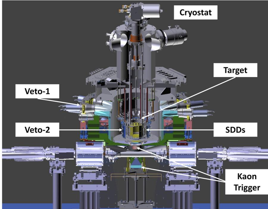
Figure 2: *Schematic view of the SIDDHARTA-2 setup.*
