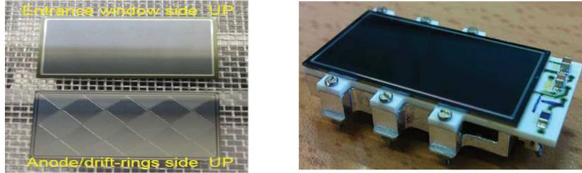
Figure 1: *The new 2 x 4 SIDDHARTA-2 SDDs array together with the readout electronics.*
