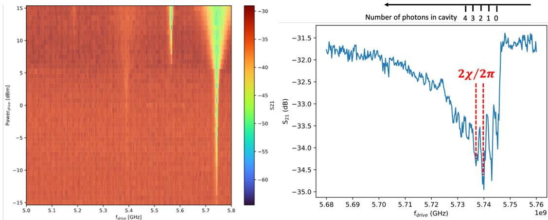
Figure 2: Left: two tone spectroscopy where we acquired the dressed cavity transmission as a function of the power and the frequency of the drive tone. Different absorption peaks are clearly observable from which we estimate the anharmonicity  $\alpha/2\pi = 353$  MHz. Right: Qubit spectroscopy of individually resolved photon numbers inside the cavity ( $P_{probe} = -122$  dBm). Each peak is separated by  $2\chi/2\pi = -2.4$  MHz.
