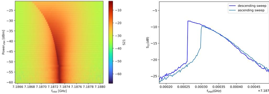
Figure 7: *Left*: Resonator spectroscopy as a function of the readout power. The dressed cavity frequency shows strong non linear behavior. *Right*: Transmission of the dressed cavity showing a step-like resonance and a clear hysteresis depending if the readout frequency sweeps from low to high values (ascending) or vice versa (descending).
