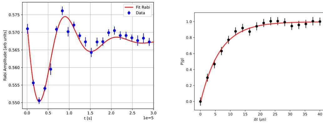
Figure 9: *Left*: Rabi oscillations of the VdW qubit. Spectrum acquired with drive frequency 12.611 GHz and power -167.7 dBm. *Right*: Measurements of the relaxation time  $T_1$ . From fitting procedure (red line) we estimate a  $T_1 = 6.5 \pm 0.4 \mu\text{s}$
