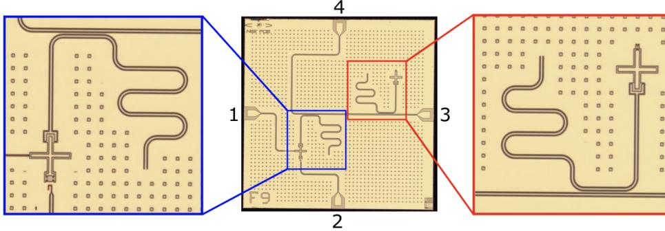
Figure 3: Optical image of the 2 qubit device. On the left we reported a zoom of the tunable frequency qubit, on the right of the fixed frequency qubit.
