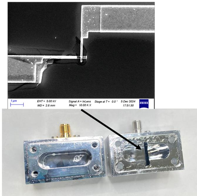
Figure 1: Picture of the qubit inside the 3D cavity and Scanning electron microscopy of the Al transmon. The image is magnified 10000x.
