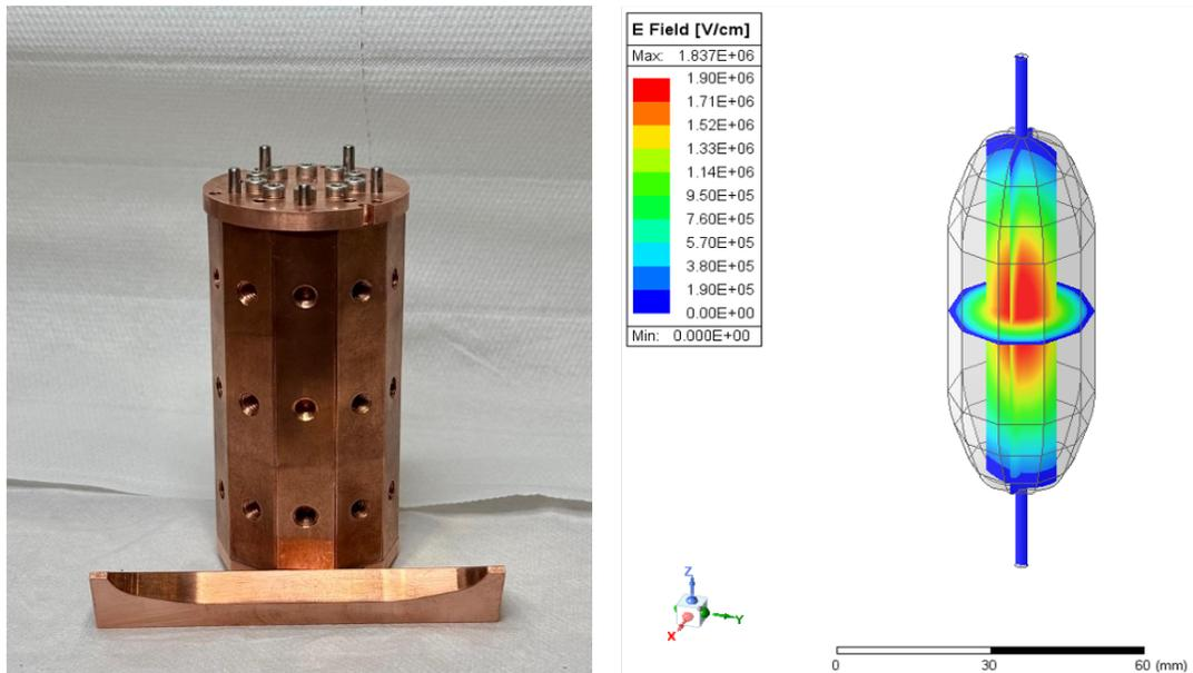
Figure 5: *Left*):10 faces OFHC Cu cavity. *Right*): ANSYS simulation of the TM 101 mode  $f = 8.489$  GHz.
