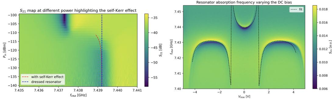
Figure 4: Left: Resonator spectroscopy as a function of the readout power. Right: frequency of the resonator-qubit dressed system as a function of the voltage bias (i.e. the frequency of the qubit). An avoided crossing is observed when the resonator and the qubit have the same resonance frequency.
