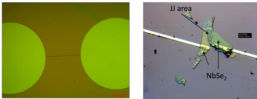
Figure 6: *Left*):optical image of the circular Al pads .*Right*): Optical image of the NbSe<sub>2</sub> JJ we used as a qubit.
