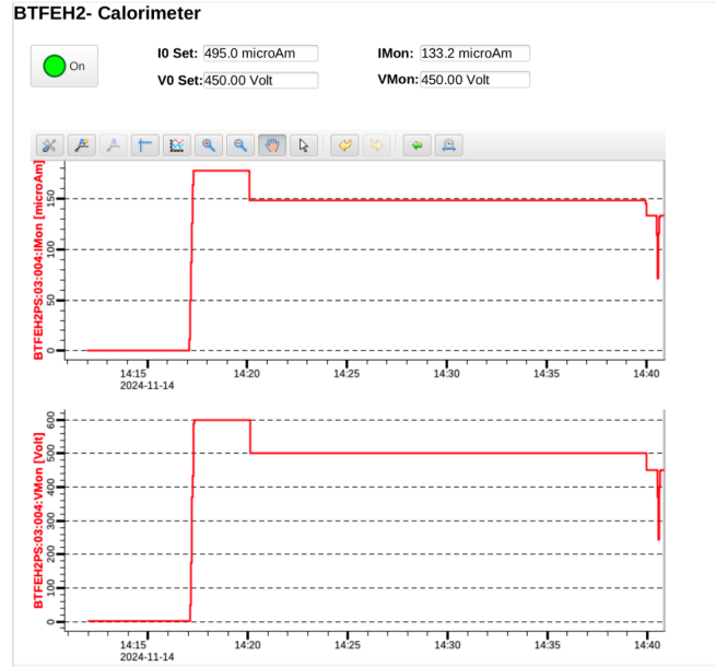
Figure 10: Phoebus interface for CAEN HV power supply control
