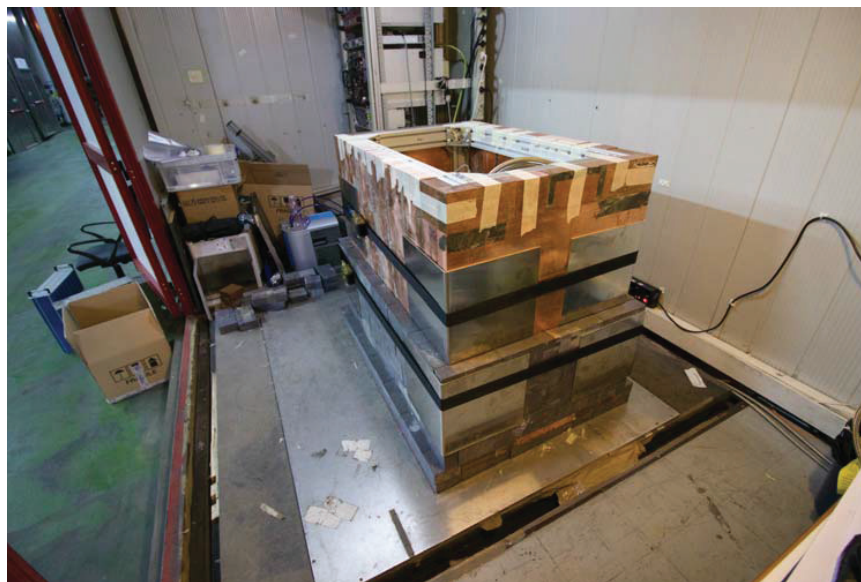
Figure 4: The VIP-2 shielded setup at LNGS, during installation (upper part here is still to be installed).
