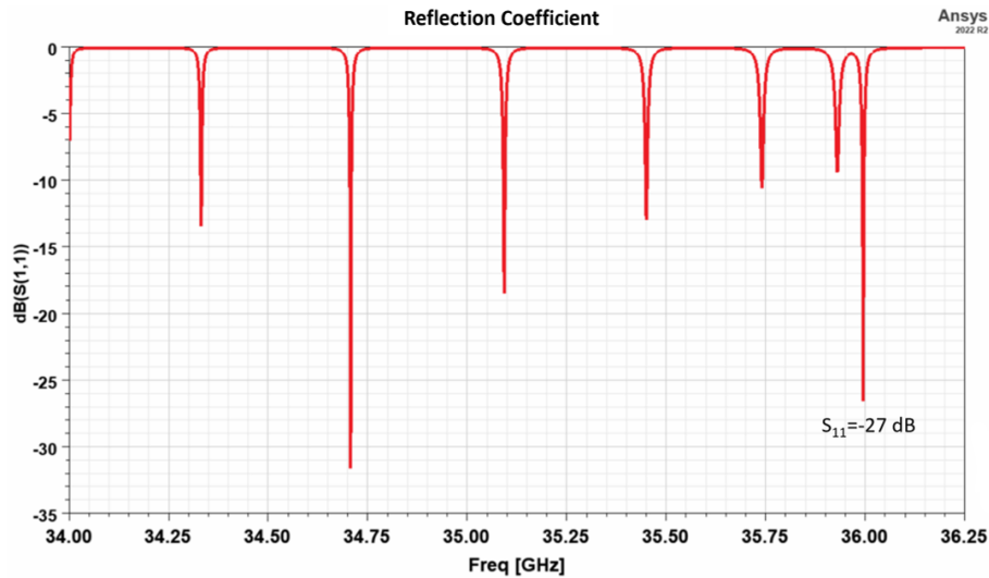
Figure 2: Reflection coefficient, S_{11} , at the input rectangular port of the waveguide of the mode launcher.
