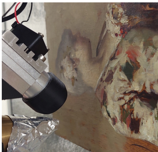
Figure 4: The XRF system being placed, using the ARTEMISIA scanner, nearby the Favretto's painting to start the atomic mapping.
