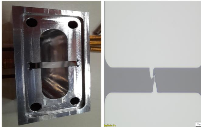
Figure 1: **(Left)**: Al cavity hosting the transmon chip. **(Right)**: optical image of the transmon shunt capacitance pads acquired with a 50 $\times$  magnification. The JJ is located between the pads.
