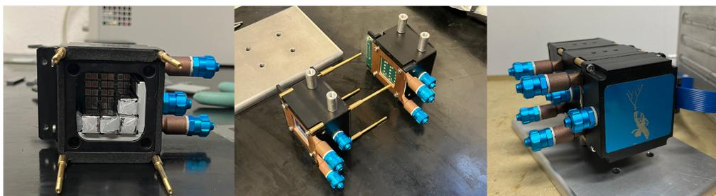
Figure 2: Proto-1 images: a single module during crystal (with a Mylar wrapping) installation, the locking system of the two layers together with the heat exchanger and finally the prototype fully assembled.
