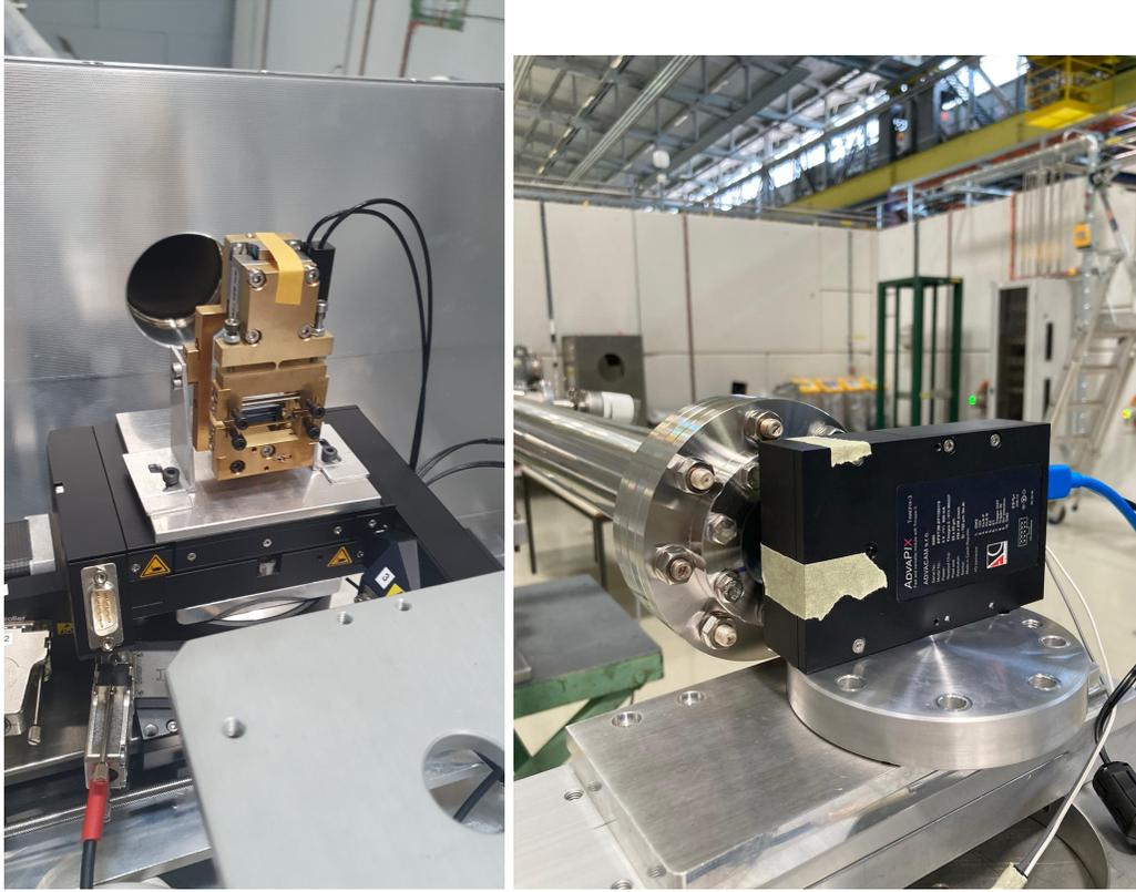
Figure 5: *On the left the Silicon crystal  $\sim 15 \mu\text{m}$  thick bent by its holder, mounted on the 3-axis handling system and centered on the 0.5 GeV positron beam axis. On the right the TimePix3 detector positioned at the end of the T9 beam line, 3 m downstream the bent Silicon crystal. The TimePix3 is positioned in air, just downstream a Mylar window  $50 \mu\text{m}$  thick that closes the beam pipe.*
