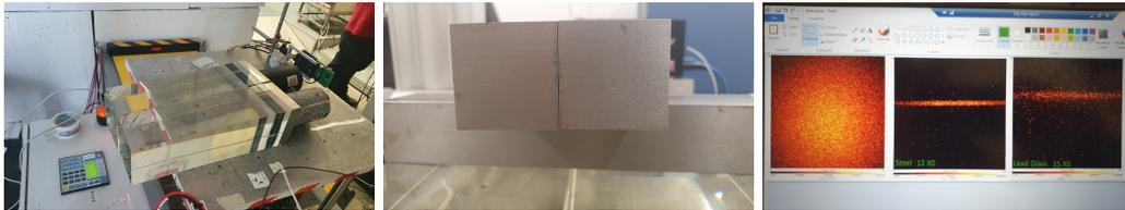
Figure 4: *On the left the lead-glass collimator. In the center the iron collimator. On the right the TimePix3 pictures of the beam without collimators, with iron collimator and lead-glass collimator respectively ( $\sim 0.15$  mm gap).*
