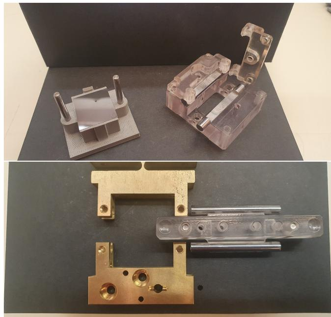
Figure 2: *Up on the right the seat for the silicon crystal during the gluing, on which the support for the crystal bending pins (up on the left) is clamped. The glue is deployed on the two pins before superimpose them on the crystal. Then, the crystal glued on its pin is clamped in a dedicated “sandwich support” used to insert it in the two brass forks of the bending holder.*
