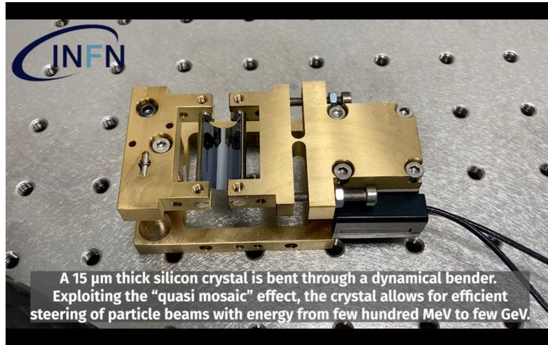
Figure 1: *Crystal active bending holder. The bent silicon crystal plate, in between the two brass forks, is bent by the horizontal movement of one of them by the piezo motor.*
