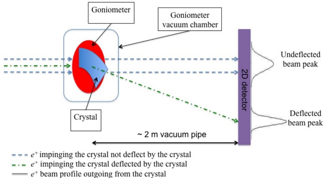
Figure 3: *SHERPA BTF apparatus scheme.*
