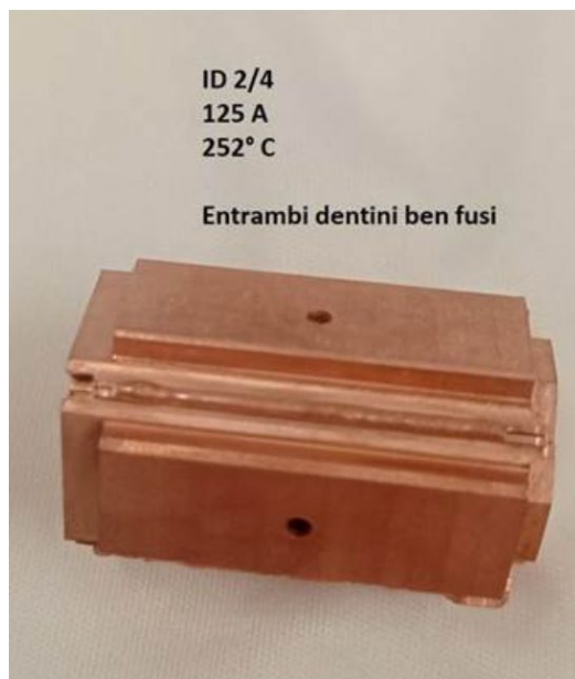
Figure 6: Four-quadrant cavity after TIG welding.
