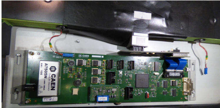
Figure 3: Picture of the FE card and RO board prototypes installed inside a Top Tracker module.
