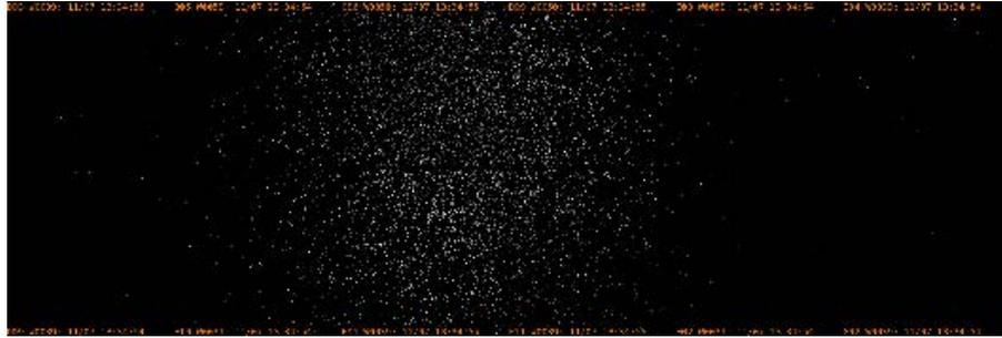
Figure 5: *Beam spot picture resulting from ToT measurements performed with Timepix3 detector.*
