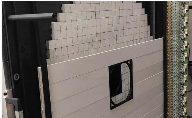
Figure 4: *The PADME lepton tagger detector (ETag) being assembled in front of the BGO calorimeter (ECal).*
