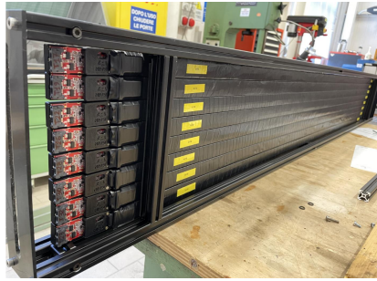
Figure 15: Pictures of one CRT module with the PVC light-tight box removed.
