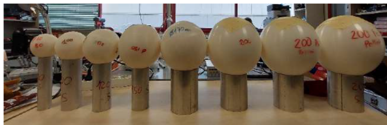
Figure 5: Bonner spheres of the SAMADHA spectrometer.
