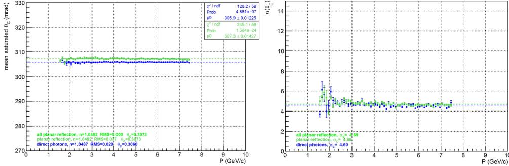
Figure 9: Comparison between the Cherenkov angle mean for photons with no reflections (blue points) and those with one reflection on one of the lateral mirrors (green points) as a function of the momentum. The left plot show the mean of the distributions and the right one the sigma. Data for electrons and negative pions.
