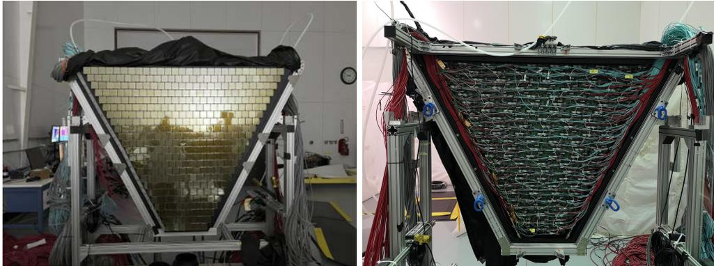
Figure 2: *The RICH electronic panel from the MAPMT (left) and front-end (right) side.*
