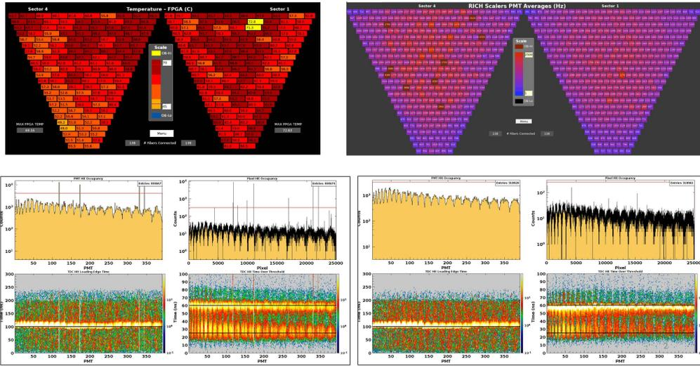
Figure 8: *RICH monitoring plots during normal CLAS12 data taking: FPGA temperatures (top left), scaler readout counts per MAPMT (top right), TDC readout counts and time distributions per MAPMT and per channel (bottom).*
