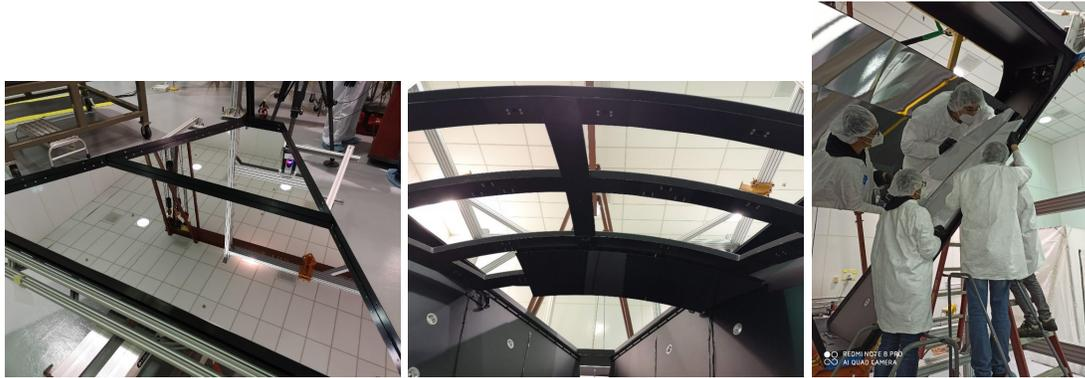
Figure 5: *Phasis of the assembly of the mirrors: the frontal mirrors (left), the spherical mirrors (center), the lateral mirrors (right).*
