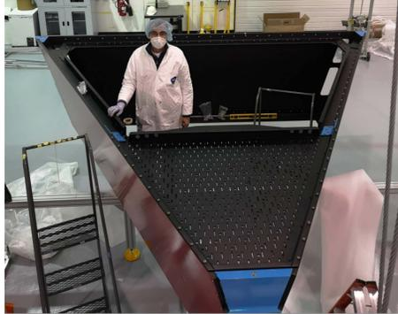
Figure 1: *The RICH external frame fully assembled.*
