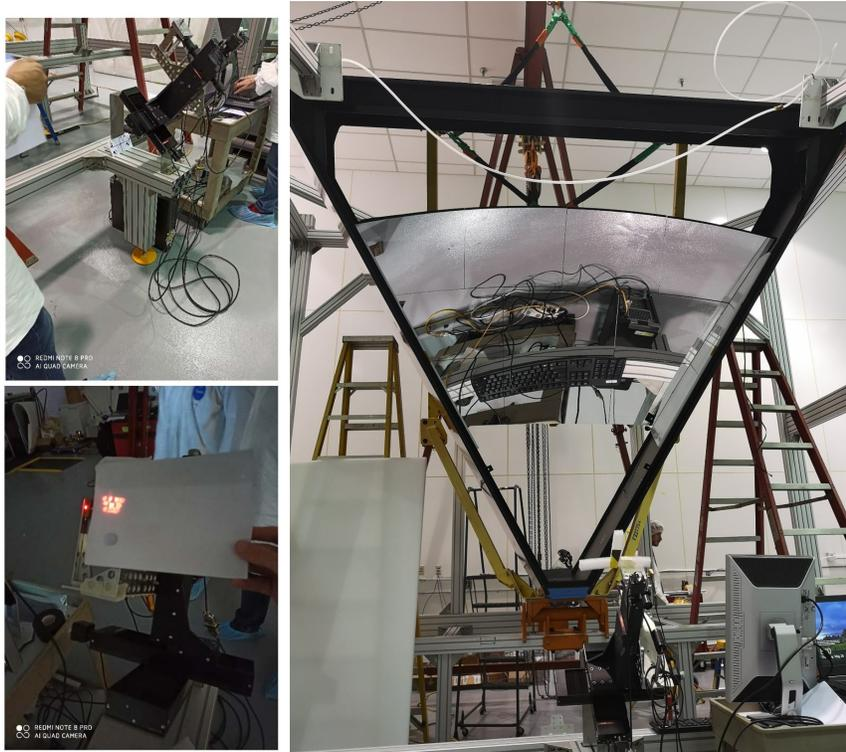
Figure 6: *The setup used for the spherical mirror alignment (top left), the reflected spots before the alignment (bottom left) and mirror after the alignment (right).*
