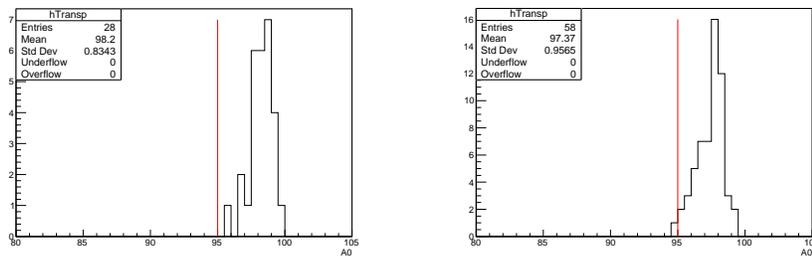
Figure 3: *Transparency of the aerogel tiles with 2 cm (left) and 3 cm (right) thickness.*
