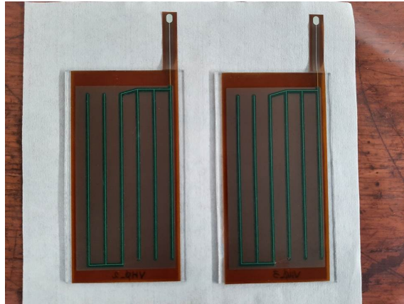
Figure 18: DLC-HR electrodes. DLC resistivity is 7 \text{ G}\Omega/\square , grid pitch 1 cm.
