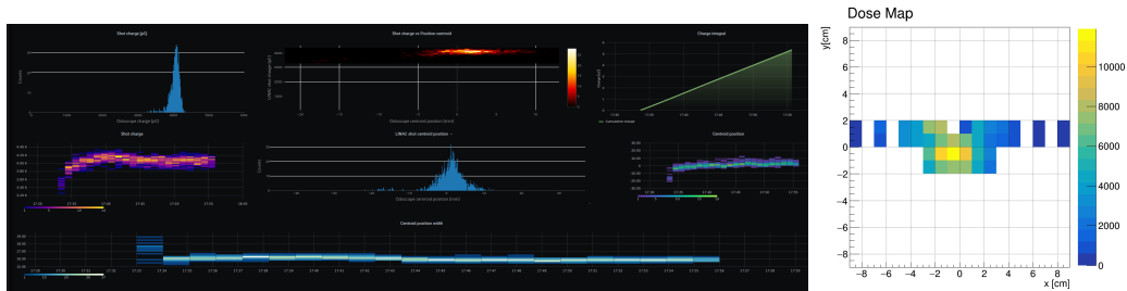
Figure 7: Left: Improved Control dashboard realized to monitor the beam parameters distributions (charge and position) while the LINAC is normally operated for injection in the DAFNE Main-Rings. This tool allows online information on the beam spot on the target and thus estimates, on the basis of the calibration, of the expected dose in the irradiation site. Right: radiation field dose map after the odoscope lead shielding. Dose is measured in mGy. ( Data courtesy of LNF radioprotection service )
