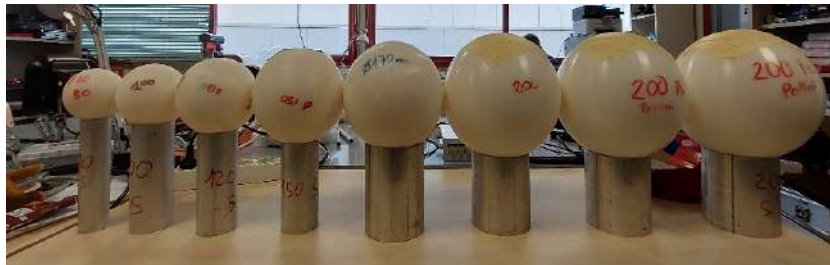
Figure 2.1. Bonner spheres of the SAMADHA spectrometer.
