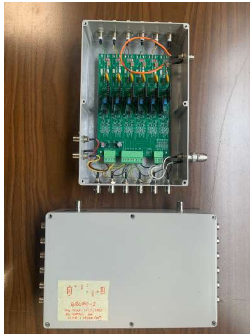
Fig. 2.6. 6-channel analogue boards.
