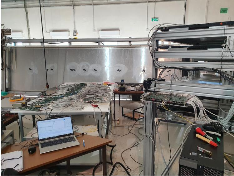
Figure 4: *RO board final prototypes tests at Strasbourg. Test bench simulation of one wall (16 FE+RO boards coupled to one concentrator) at left and detector prototype for track reconstruction at right.*
