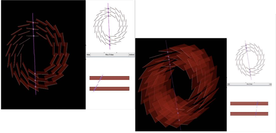
Figure 4: *Cosmic Tracks in the full Inner Barrel of the new ITS during commissioning.*
