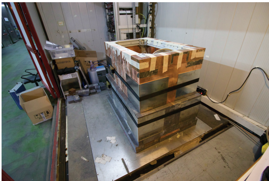
Figure 4: The VIP-2 shielded setup at LNGS, during installation (upper part here is missing).
