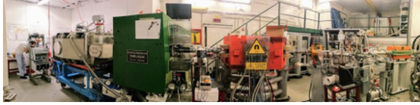
Figure 2: The DAFNE Beam-Test Facility (BTF), an overview of the 2019 layout: PADME vacuum chamber and detectors on the left, BTF2 line on the right
