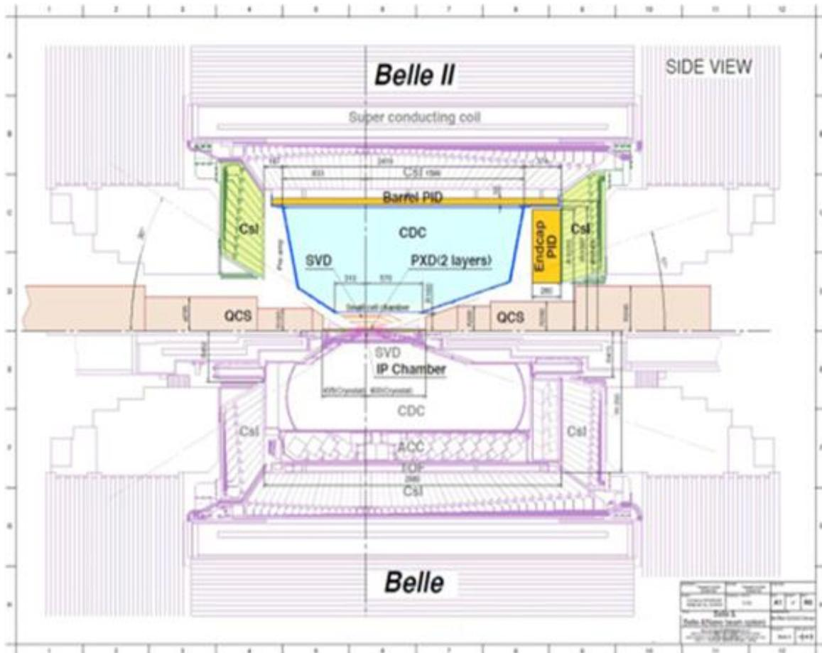
Figure 2: Comparison among the Belle (bottom) and Belle II (top) detectors. In color the upgraded parts.
