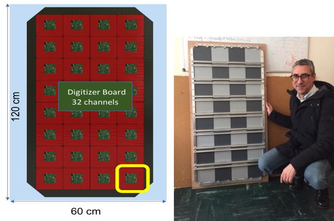
Figure 3: Left: schematic layout of a 32-tile module 0 of the muon system. Right: full-size mock-up of a module 0.
