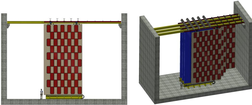
Figure 4: Left: Front view of one station of the HS muon system. Each station is made of 100 modules, 32-tile each, disposed in a chess structure staggered on both sides of a supporting wall. Right: 3D view of the HS muon system, with four active stations and three iron filters. The stations are designed to slide on rails in order to ease the access to the modules.
