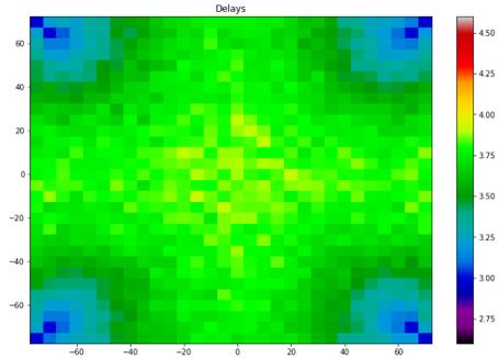
Figure 1: FLUKA simulation: time response of the analog sum as a function of different impinging points of a particle on a square  $15 \times 15 \text{ cm}^2$  tile.
