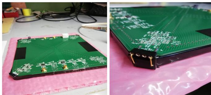
Figure 2: Left: prototype of the customized readout board for a  $(15 \times 15 \times 1) \text{ cm}^3$  square tile with four SiPMs at the corners. Right: detail of the board connection to the SiPMs.
