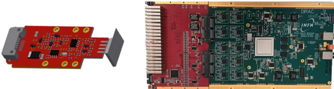
Figure 10: Left: CAD drawing of a FEE board connected to a Mu2e-SiPM. Right: Picture of Mezzanina and DIRAC boards connected together.
