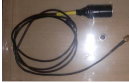
Figure 2. Collimated thermal neutron detector built for tests at INES beam-line. The sensitive capsule has diameter 15 mm and length 35 mm. The internal thermal neutron sensor has 1 mm 2 area and the collimating channel has diameter 1 mm x length 8 mm.
