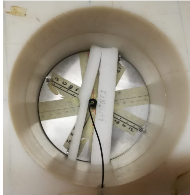
Figure 4. Position of the detector in HOTNES test point (+50 cm from the facility bottom).
