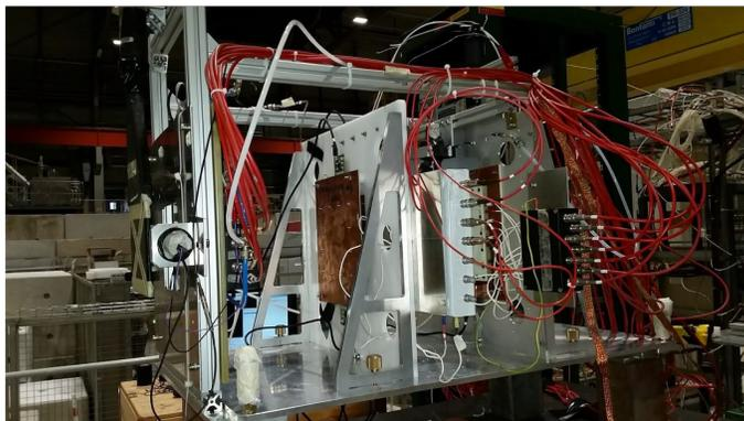
Figure 5: The  $\mu$ -RWELLS prototype coupled to the emulsion brick mounted in the H8 area of CERN SPS.
