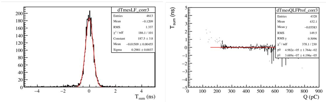
Figure 3: Intrinsic time response of the rectangular tile for a beam impinging on a central position of the tile (left) and time response dependence with the signal amplitude (right). After the subtraction of the  $T_0$  time jitter, the rectangular tile has an excellent intrinsic time resolution of  $\sim 280$  ps, with essentially no dependence on the signal amplitude.
