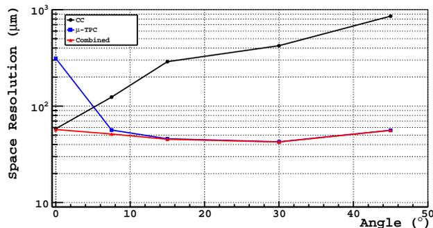
Figure 6: Spatial resolution of the  $\mu$ -RWELL as function of the track incidence angle.
