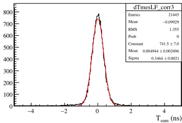
Figure 4: Time response of the rectangular tile averaged over the central points of one of the two halves of the tile. The time resolution is the convolution of the intrinsic response of the tile and the time-drift of time response distribution with the impinging point of the beam. After the subtraction of the  $T_0$  time jitter, the rectangular tile has an excellent average time resolution of  $\sim 320$  ps.
