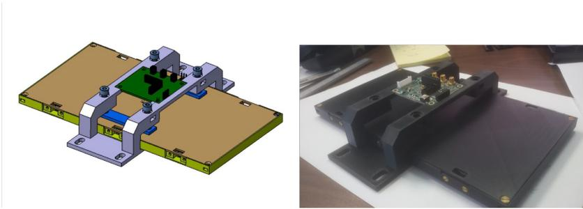
Figure 1: Design and realization of the ( $10 \times 20 \times 0.8$ ) cm<sup>3</sup> rectangular tile read out by 6 SiPM ( $6 \times 6$ ) mm<sup>2</sup> and the ASIC chip MUSIC, housed in the tile support.
