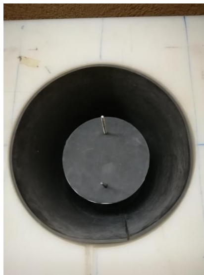
Fig. 9. EPI41-c Internal cavity lined with borated rubber and EPI41-c epithermal filter covered with
