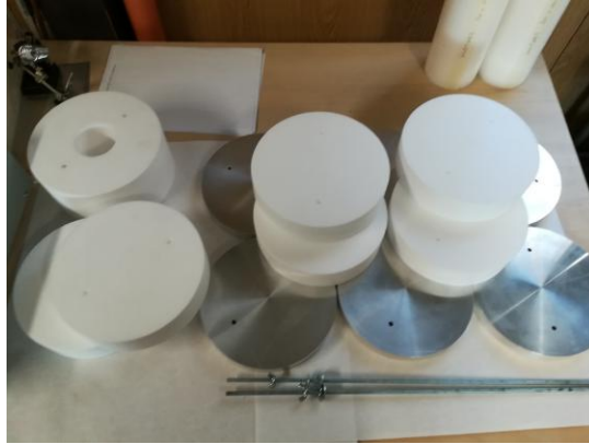
Fig. 7. Aluminium and Teflon disks (2.5 thickness, 20 cm diameter).
