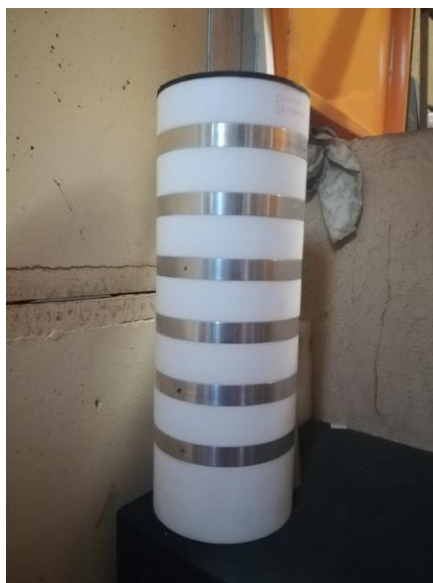
Fig. 10. Parts of Teflon and Aluminium used to assembly the EPI41-c epithermal cavity.
