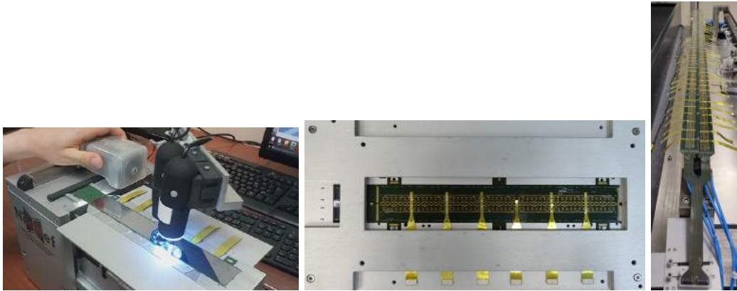
Figure 3: Left: an OB HIC at the reception test. Center: the HIC is contained in a carrier plate which allows transport, storage, powering, testing, and vacuum gripper placement for handling. The left side of the HIC shows the so-called “tab” used to connect the sensors to the readout system. Once the HIC is qualified for alignment and gluing, the tab has to be cut. Right: the two HS assembled in a stave: the sensors are glued directly on the carbon fiber strips. The blue pipes are the embedded water cooling lines (input and output). The HS are read-out by soldering an extension tab which is the interface with the outside world of the 98 ALPIDE chips. It can be clearly seen that the two HS come in different flavors (upper and lower) which have a partial longitudinal overlap requiring a definite sequence of installation.
