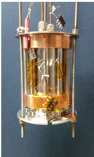
Figure 3: Nb cavity instrumented before the insertion in the LHe criostat.
