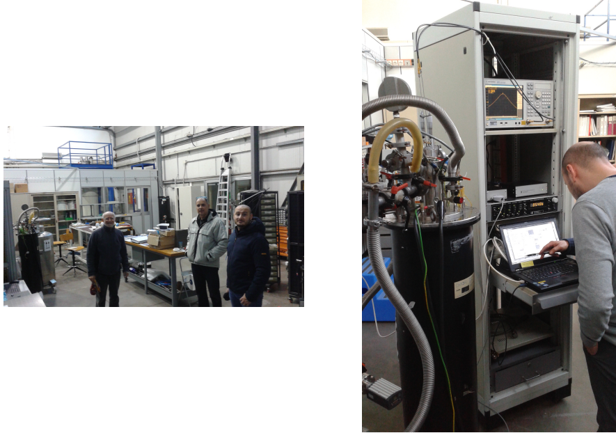
Figure 2: Left: The new COLD laboratory in building 8. Right: The LHe cryostat and DAQ and measurement system of the Quax resonant-cavity after moving in the COLD laboratory.
