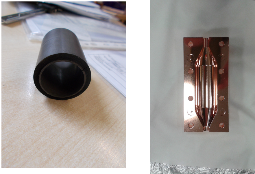
Figure 6: Left: The two resonant cavities that will be tested in 2018: (left) MgB2 cavity; (right) NbTi cavity.
