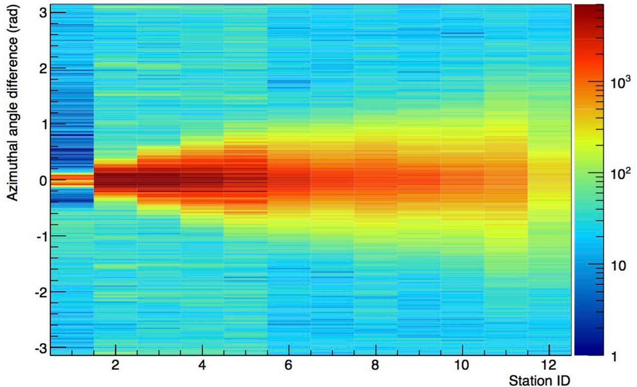
**Figure LAV-1.** Distribution of difference in azimuth,  $\Delta\phi$ , between clusters on different stations vs. the number of stations between the most upstream and downstream clusters.
