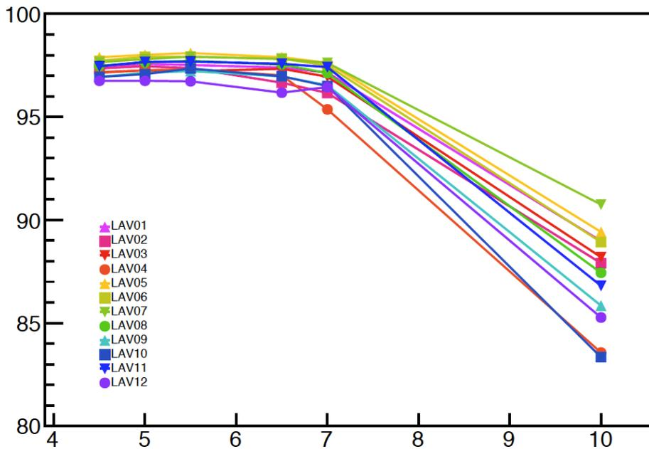
**Figure LAV-2.** Average MIP detection efficiency for different stations as a function of threshold.
