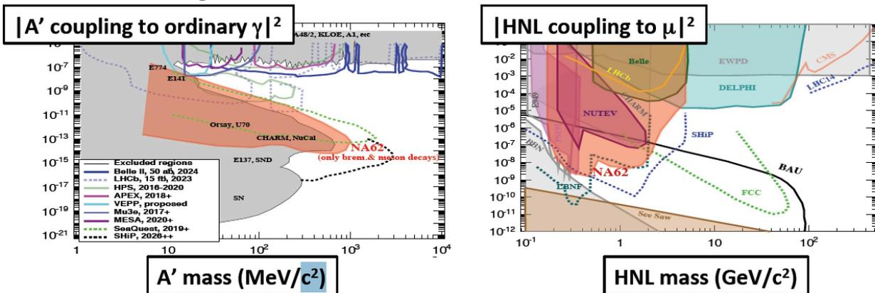
Fig ana-2-3: 90%-CL upper limit in the  $e2$  vs  $M$  plane for dark-photon (left) and heavy neutral lepton (right)
