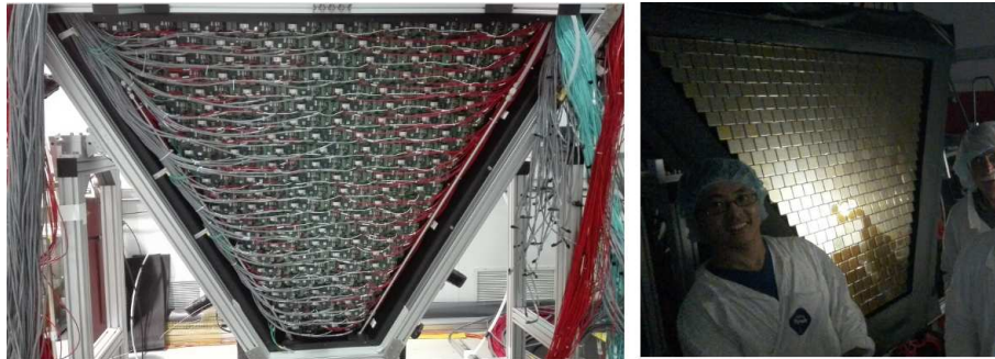
Figure 10: The electronic panel from the MAPMT (left) end readout electronics (right) side.
