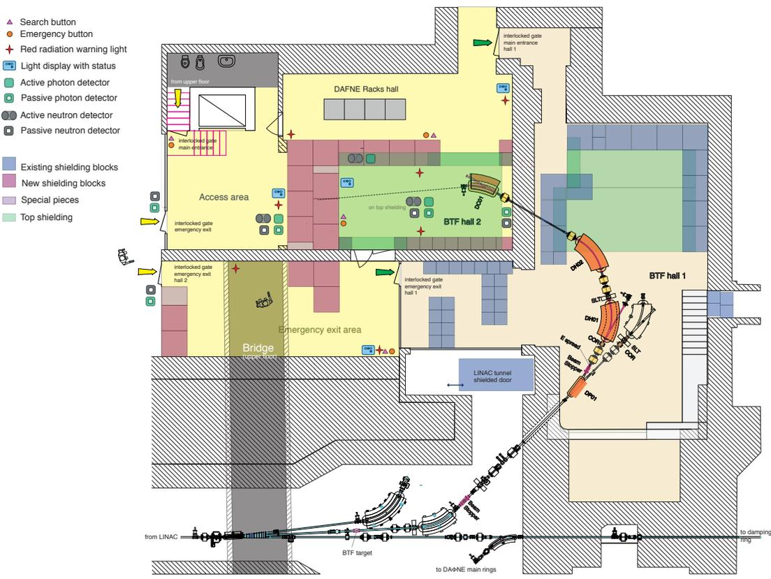
Figure 2: *The new BTF layout with two beam-lines and two experimental areas.*
