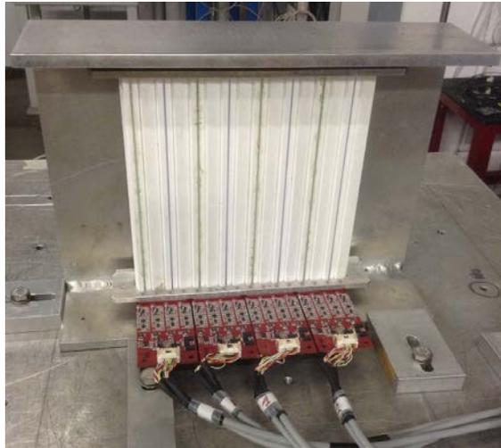
Figure 8: *The charged particle veto prototype placed on the BTF table and prepared for tests.*
