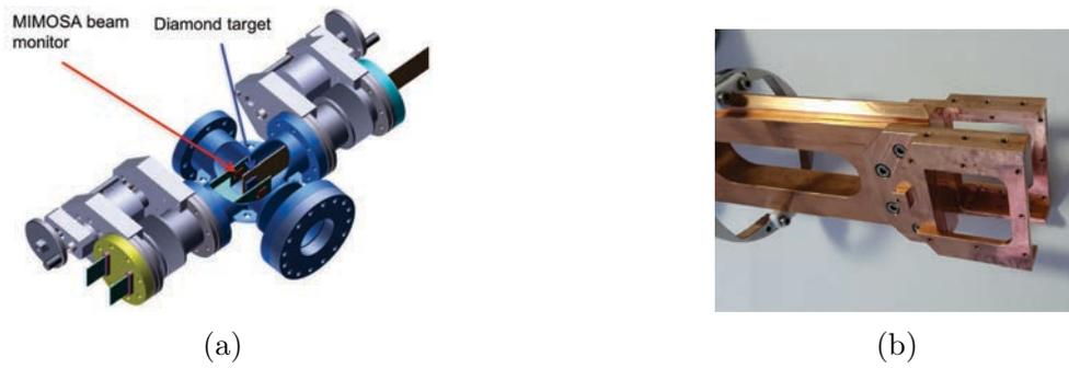
Figure 11: (a) Mechanical layout of the Target region. Two step motors can insert in and out of the beam line both the target and the silicon beam-monitoring system. (b) Mechanical holder of the MIMOSA monitoring system (realized by LNF mechanical workshop).
