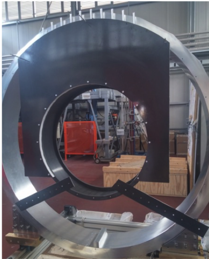
Figure 11: Full size mock-up of the calorimeter mechanical structure.
