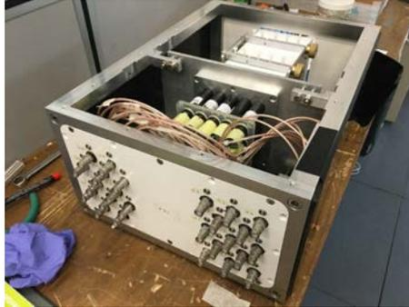
Figure 5: *Layout of the PADME main e.m. calorimeter prototype. It consists of a matrix of 25 BGO crystals on which different photosensors can be mounted for tests.*
