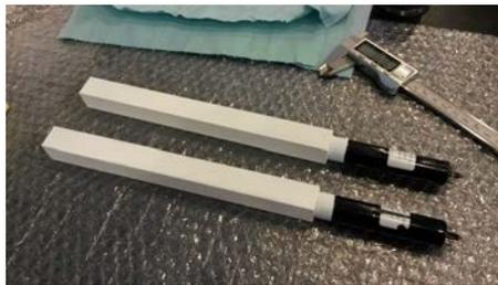
Figure 4: *Two elements of the PADME main e.m. calorimeter. The dimensions of the BGO crystals are  $20 \times 20 \times 230 \text{ mm}^3$ .*
