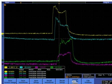
Figure 9: *Bunch length measured at different points of the DAΦNE LINAC during the tests to extend bunch duration. A length of 250 ns has been reached (yellow curve) at the end of the line.*
