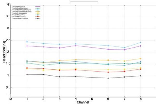
Figure 8: *Estimated time resolution (in ns) for the different scintillator slabs. The different lines represent different evaluation methods (see test for more details).*
