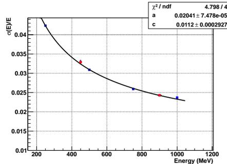
Figure 6: *Energy resolution measured with a prototype of the PADME ECAL at the LNF BTF. Red and blue points refer to two different beam energies of 450 and 250 MeV, respectively. The line is the best fit curve whose parameters are quoted in the inset.*
