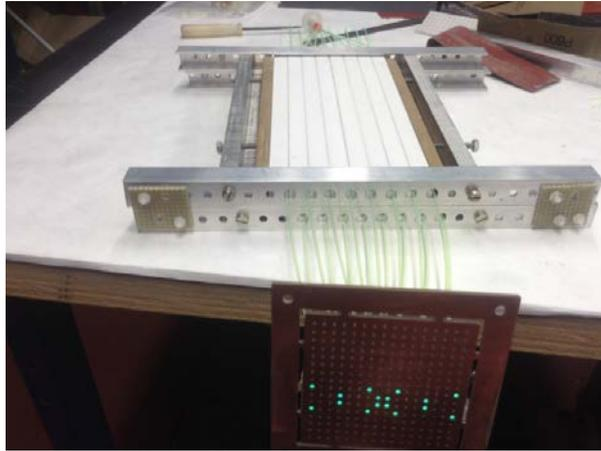
Figure 7: A picture of the double layer prototype of the charged particle veto before coupling it to the multianode PMT.
