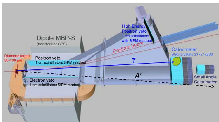
Figure 1: *PADME detector layout. From left to right: the active target, the positron/electron vetoes inside the magnetic dipole, the high energy  $e^+$  veto near the non-interacting beam exit, the e.m. calorimeters. The distance from the target to the first calorimeter is roughly 3 m.*
