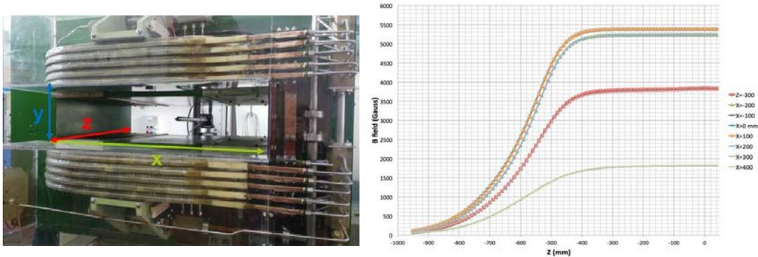
Figure 3: **left** the PADME magnet. **right** Longitudinal scan of magnetic field at different transverse positions.
