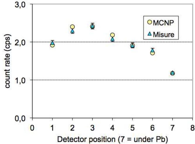
Figure 3: Observed and expected count rates in the CYSP-HS detectors, when the device is exposed in a reference  $^{241}\text{Am-Be}$  neutron field (Politecnico di Milano).
