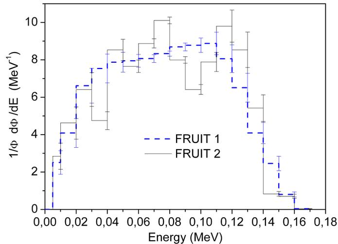
Figure 7: Neutron spectrum obtained by unfolding the CYSP-HS data with FRUIT. FRUIT 1 and FRUIT 2 refer to different "guess spectra" used to start the unfolding process.
