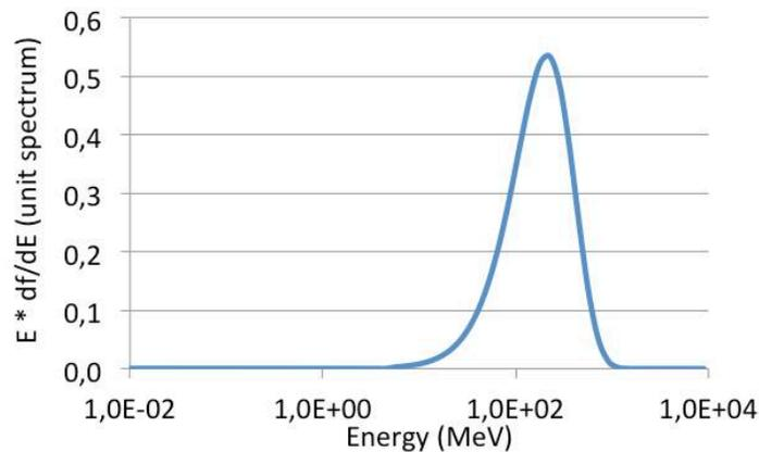
Figure 6: Typical cosmic neutron spectrum obtained by unfolding the CYSP-HS data. The spectrum is normalized to unit fluence and in equi-lethargy representation.
