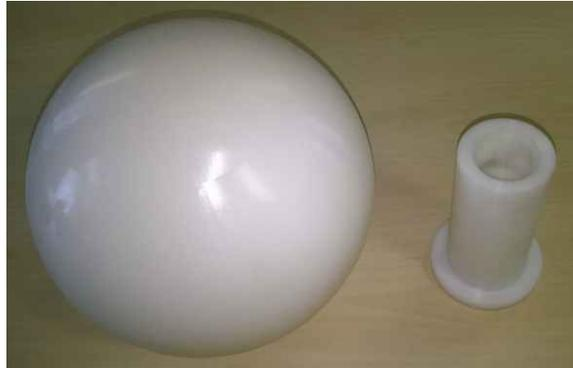
Figure 8: The SPEEDY detector, made of a 22 cm diameter sphere, and the detector cylindrical insert (detector cavity: 4 cm height x 4 cm diameter).
