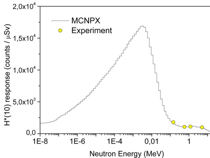
Figure 9: SPEEDY Response function in terms of ambient dose equivalent  $H^*(10)$ : simulated values (curve) compared with experiment with mono-energetic neutrons at few neutron energies.
