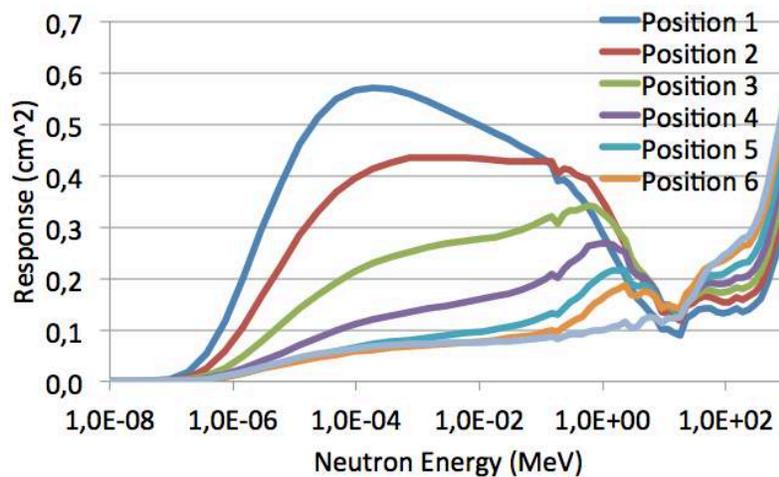
Figure 2: CYSP-HS response matrix (counts per unit fluence as a function of energy and detector position).
