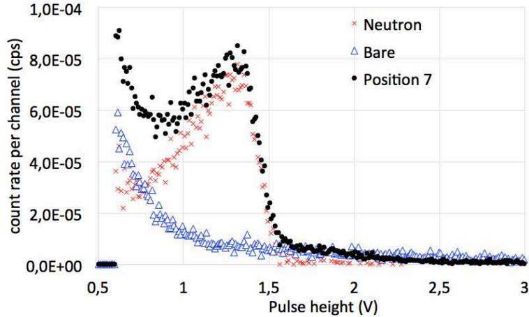
Figure 5: Typical pulse height spectrum of the LATND located in position 7. The photon signal is obtained from the "bare" detector data. The "neutron" spectrum is the difference between the total and the photon spectra.
